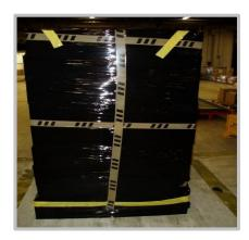
As far as possible, composite stacking must be observed when assembling pallets
